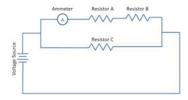
If you wanted to measure the current through resistor C, you would place the ammeter on the same branch of the circuit as resistor C. If you wanted to measure the total current in the circuit, you would place the ammeter in series with the voltage source.
