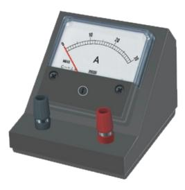
In order to measure the current that flows through a device the **ammeter must be connected in series** with the device. For example, in the circuit shown below, the ammeter is measuring the current through Resistor A and Resistor B (all 3 are in series), but not through Resistor C (not in series).
